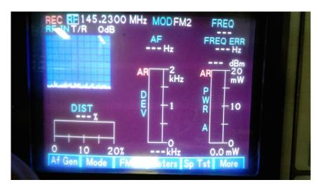
With 38 Watts of RF being applied to HP (Tx) branch, there is less than 0.0 mW of RF making it through the LP (Rx) branch.
