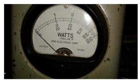
No detectable R.F. power being reflected from the branch back to the transmit radio. SWR is excellent.
