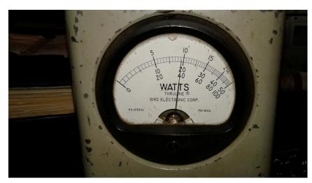
38 Watts of RF power being applied to HP branch (145.230 MHz Tx Branch.)
