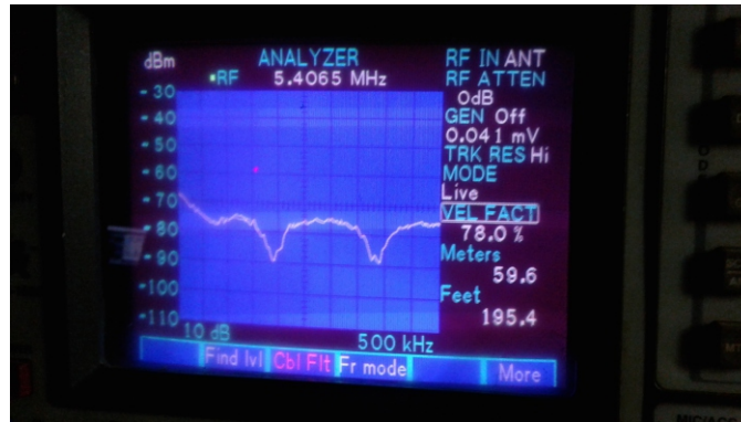
IFR-1500S semi-automatic "Fault" function measures cable length as 195.4 feet, based on 0.78 Velocity Factor (VF).
