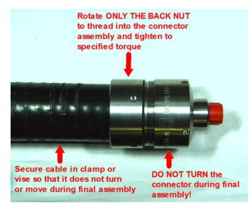
Lacking the availability of the spanner wrench and adapters, there was no feasible means of using a torque wrench to tighten the back nut to the connector body to the factory specified torque. In deciding how tight to tighten it using the rubber strap wrenches, my logic was pretty simple:
