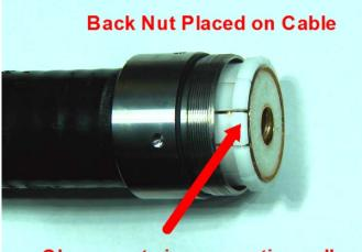
As can be seen in this photo, the Trim Tool removes exactly 1.5" inches of the cable outer jacket, and the remaining outer jacket ends on a ridge as it should for proper installation of the NF-LCF158-D01 connector. Using the proper Trim Tool eliminates the steps of overcutting the outer jacket, applying the saw guide, and cutting the outer shield, foam, and inner conductor to 1.5" length.
