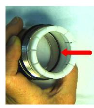
When putting the back nut on the cable, watch to make sure that this rubber o-ring sealing gasket does not get knocked out of its groove/seat in the plastic clamping assembly
