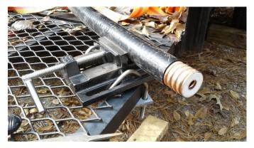
Drill press vice temporarily attached to trailer tailgate to secure cable during termination. Obviously, the spool of cable could not be just picked up and taken inside to the workbench.
