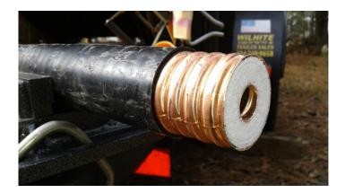
With the cable secured in the vise, the end of the cable was sawed as squarely on the end as possible. Then the RFS Trim Tool (attached to a cordless drill) was used to trim the cable. The Trim Tool is designed so that it will cut the end of the cable with the largest diameter of a ridge being the end/working face of the cable.
