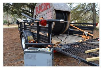
Using the highly trusted and versatile IFR-1600S as a tracking generator in order to "sweep" the LCF158 1-5/8" cable, starting from the freshly installed N-connector.
